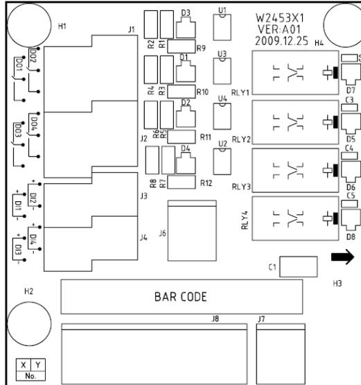
Figure 2-15 W2453X1 user interface board interface
