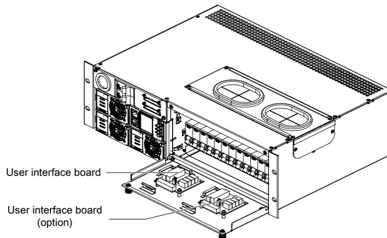
Figure 2-14 User interface board illustration of the NetSure 531 A31-S1 power system
