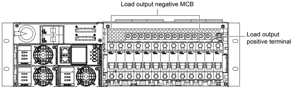
Figure 2-10 Illustration of the load cable connection terminal of the NetSure 531 A31
