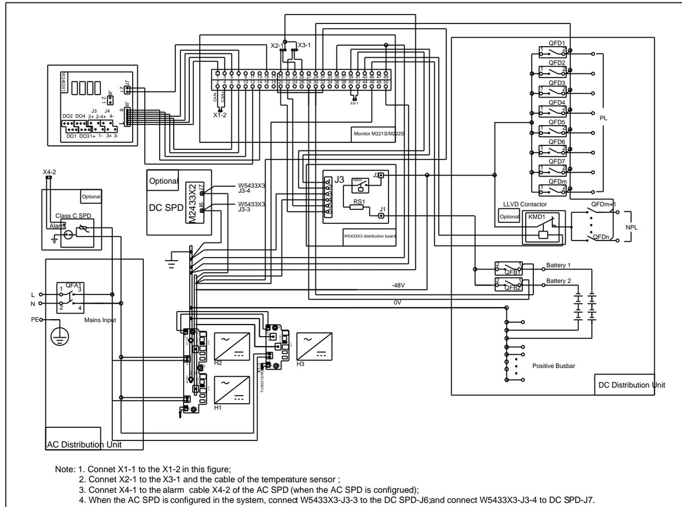
Figure 13 Schematic diagram of NetSure 531 A31-S1
