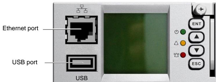
Figure 2-21 M820B controller communication port
