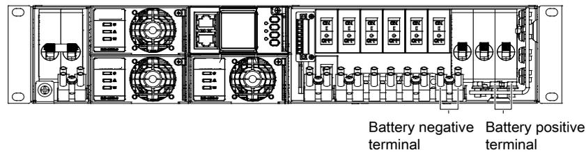
Figure 2-13 Illustration of the battery connection terminal of the NetSure 531 A32
