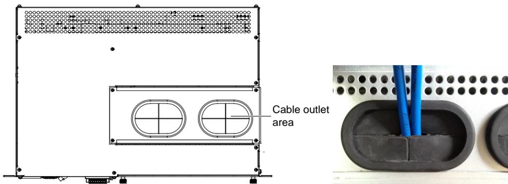
Figure 2-5 Top cable entry illustration of the NetSure 531 A31
