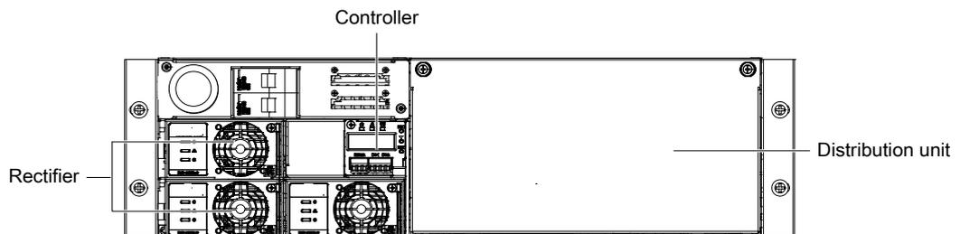
Figure 1-3 NetSure 531 A31- S3 system structure
