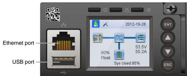
Figure 2-22 M830B controller communication port
