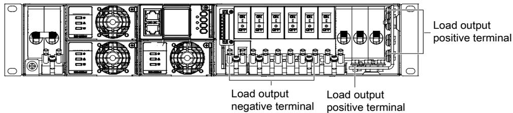
Figure 2-11 Illustration of the load cable connection terminal of the NetSure 531 A32
