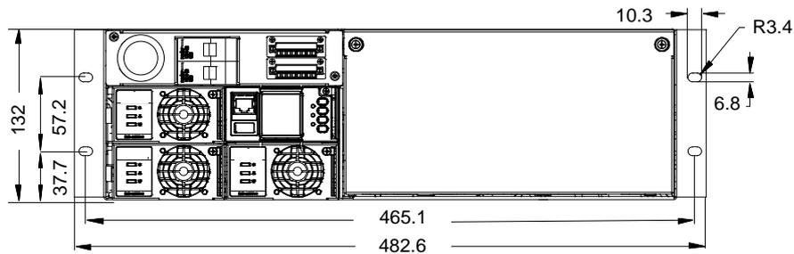
Figure 2-3 Installation size of NetSure 531 A31-S1/S2/S3 (unit: mm)
