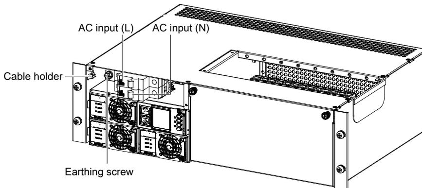
Figure 2-8 Illustration of the position of the AC input connection terminals of the NetSure 531 A31
