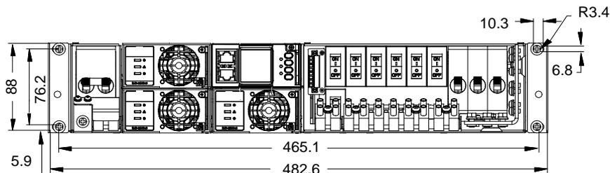
Figure 2-4 Installation size of NetSure 531 A32-S1 (unit: mm)
