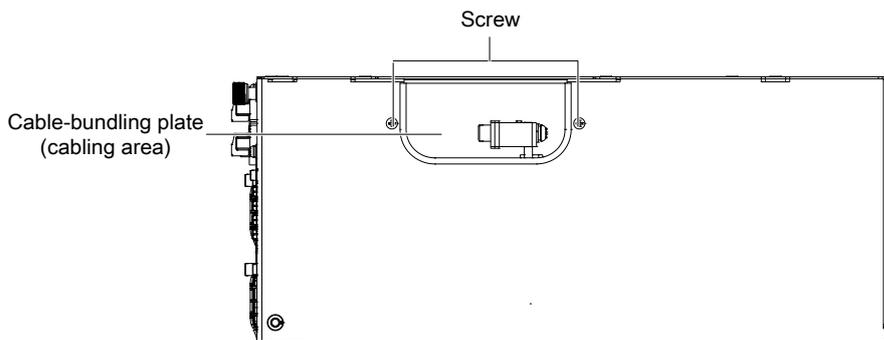
Figure 2-6 Side cable cabling Illustration
