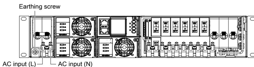
Figure 2-9 Illustration of the position of the AC input connection terminals of the NetSure 531 A32
