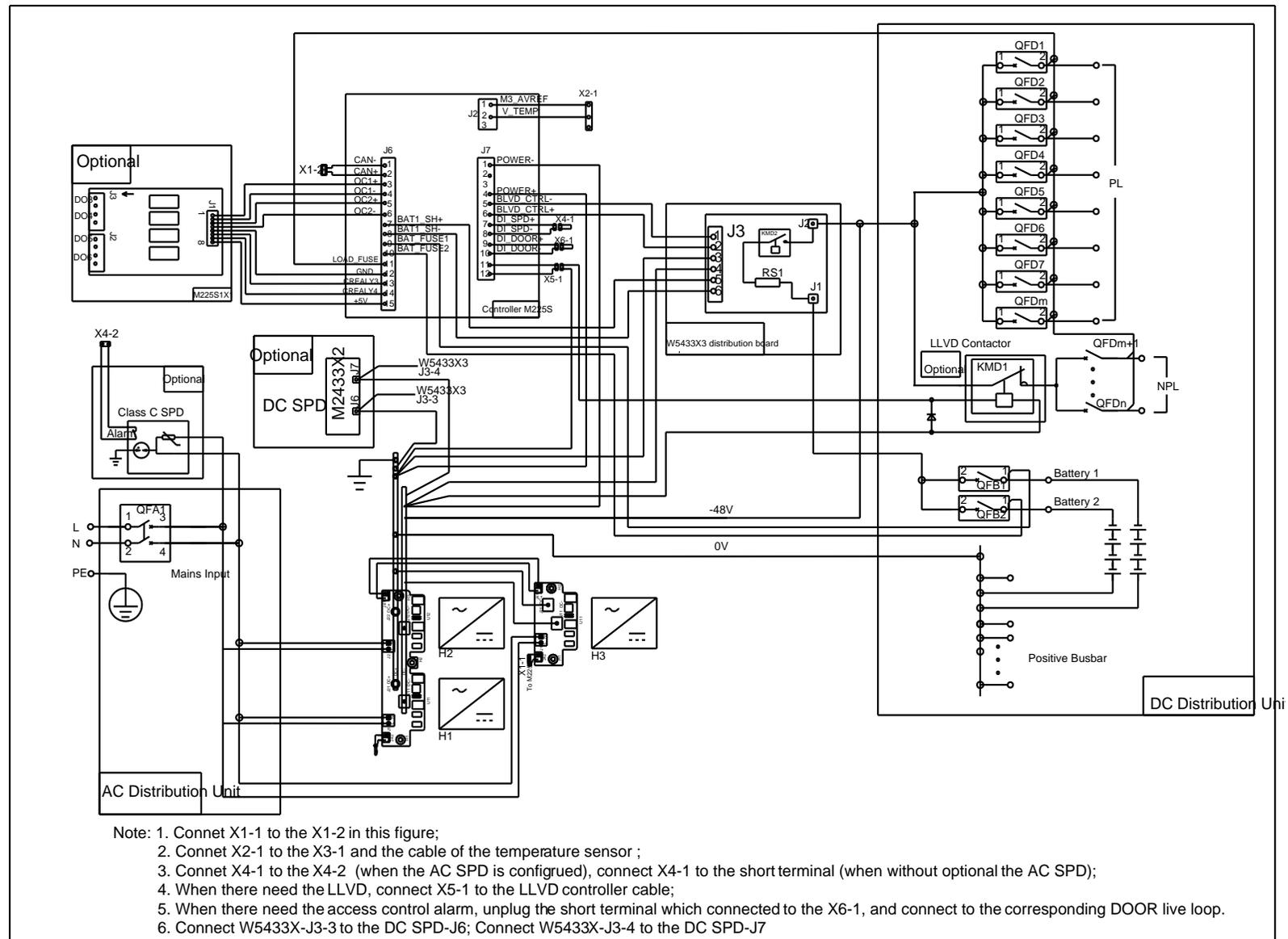
Figure 15 Schematic diagram of NetSure 531 A31-S3
