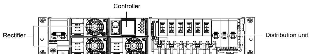
Figure 1-4 NetSure 531 A32- S1 system structure
