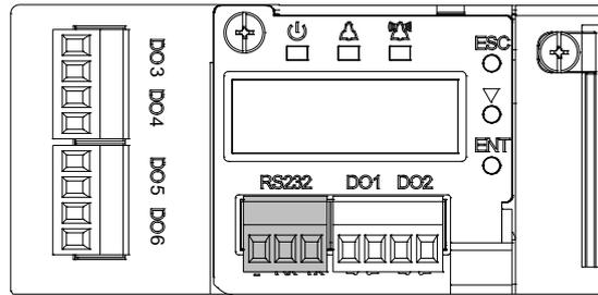
Figure 2-23 M225S controller communication port
