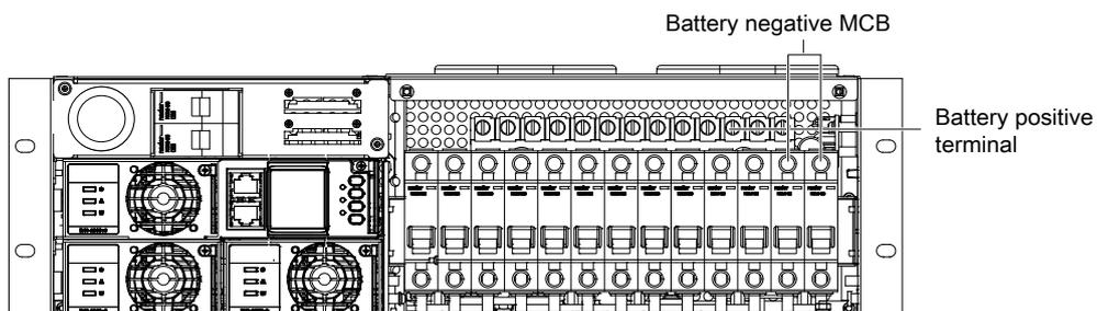
Figure 2-12 Illustration of the battery connection terminal of the NetSure 531 A31
