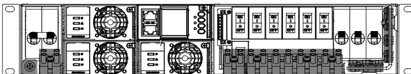
Figure 2-7 Cable cabling Illustration of the NetSure 531 A32
