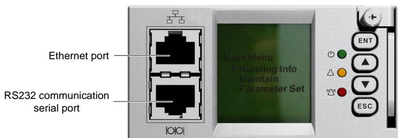
Figure 2-20 M221S controller communication port
