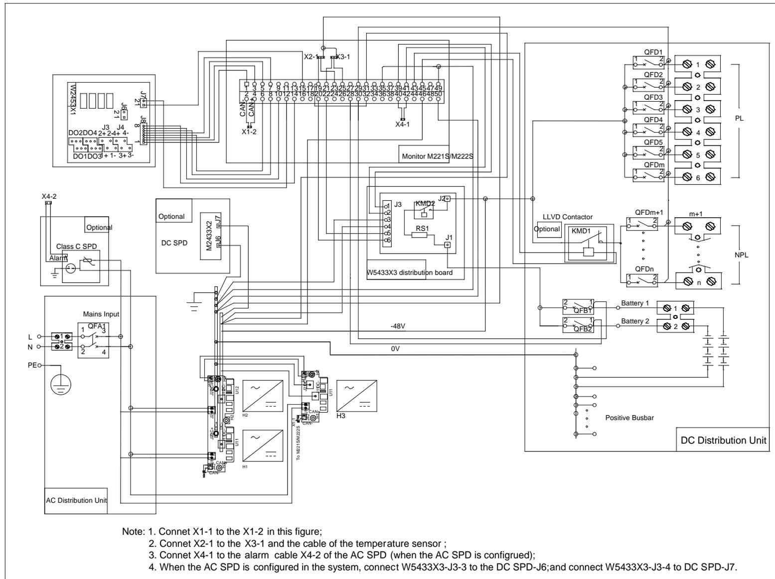
Figure 16 Schematic diagram of NetSure 531 A32-S1
