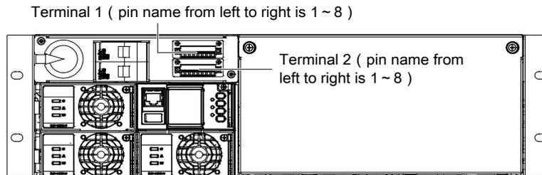
Figure 2-16 IB2 extension board port definition
