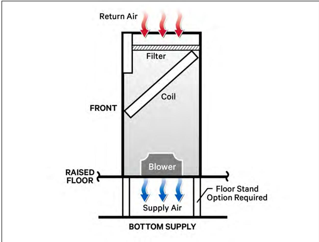
Figure 1.4 Downflow Blower Configuration, Front Air Discharge (Recommended for UPS Rooms)
