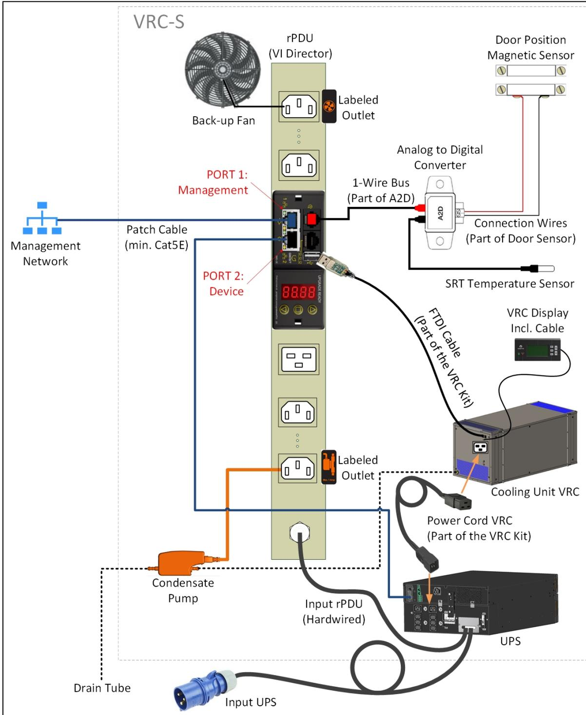
Figure 2.6 One-Line Diagram of Vertiv™ VRC-S Split Connection - EMEA (with Liebert® GXT5)
