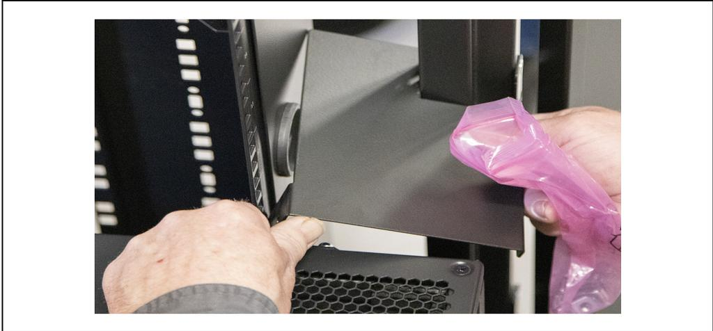
**Figure 4.3 Air Baffle Installed—800 mm (31.5 in.) Rack**
