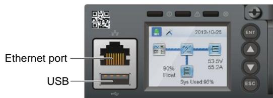
Figure 2-10 M830B controller communication port
