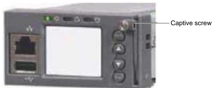
Figure 4-1 M830B Controller replacement
