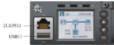
Figure 2-11 M830B controller communication port
