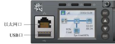
Figure 2-12 M530B controller communication port
