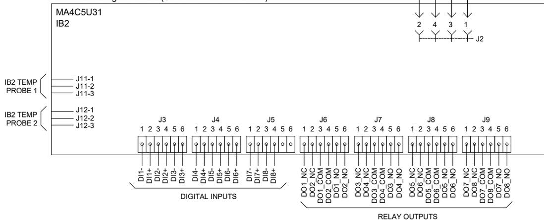
**Figure 3.6 Optional EIB (Controller Extended Interface Board) Circuit Card**
