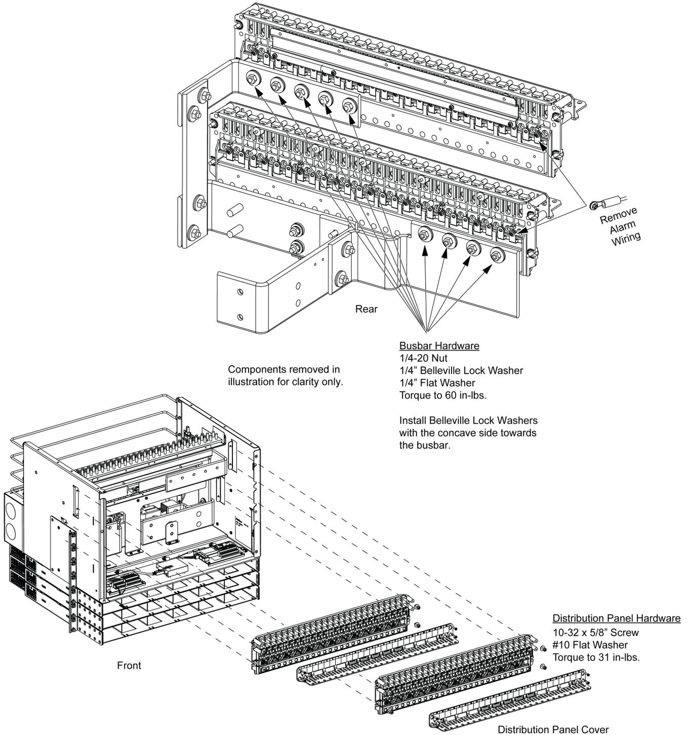
Figure 5.8: Replacing a Distribution Panel (Lists 930, 931)
