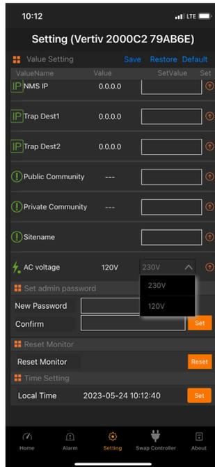
V1.00.18 and Later Versions (such as V1.10.03) Showing 120V or 230V AC Input Voltage Selection, Default at 230V, Selectable to 120V
