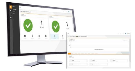
Organizations use Vertiv<sup>™</sup> Power Insight to oversee the power solutions that support their distributed infrastructure. This complimentary, web-based software provides a single interface to monitor up to 100 Vertiv<sup>™</sup> uninterruptible power supplies (UPSs) and rack power distribution units (rPDUs) and shut down critical computing resources.
