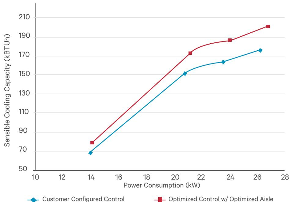
**Figure 2:** Over time, utilizing the Liebert iCOM control system with an optimized aisle configuration and control setting improves efficiency. Having those controls optimized properly by a factory-trained technician provides more capacity with similar levels of power consumption than if those controls were configured by the customer alone.
