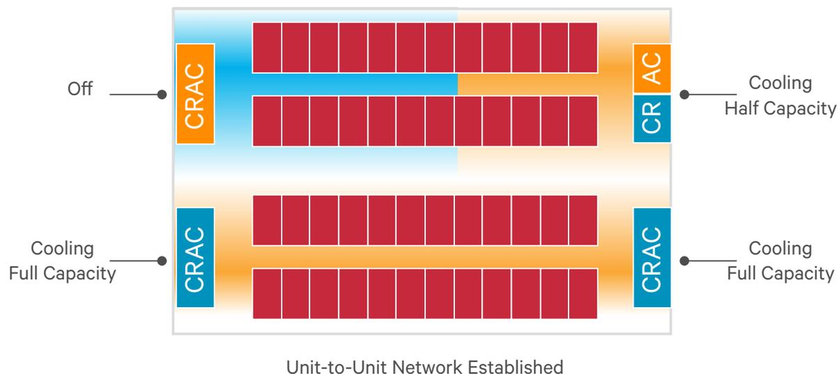
**Figure 2:** In Teamwork Mode 2, the master unit has set all units to “cooling.” However, based on varying heat loads to the units, two individual units have set themselves at “full capacity,” one at “half capacity,” and one has turned itself off.
