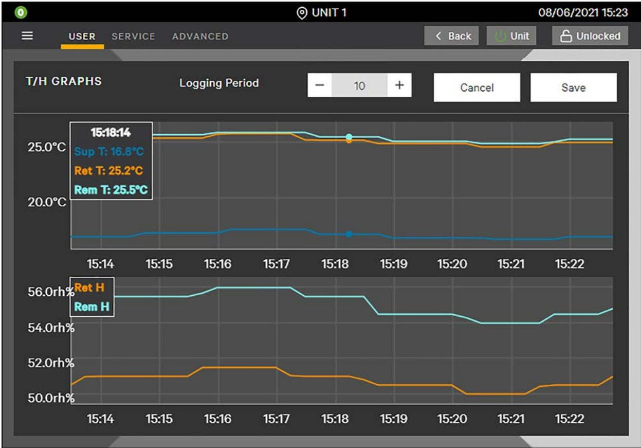
Touch the graph to display the left corner icon which will be populated with the temperature or humidity values in a timeline. The Logging Period defines the duration of logging in minutes (max 1440 minutes = 24 hours).
