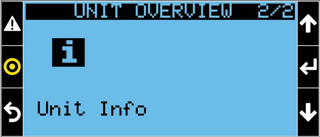
From the Main Screen, press the Decrease (⏪) Key to access the Unit Overview. A password is not required.
