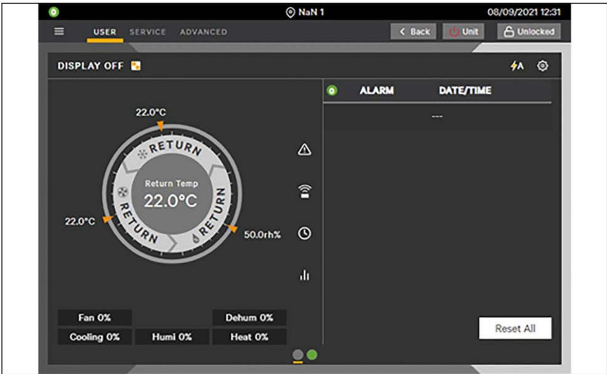
The utilization percentages of ventilation, cooling, free cooling, humidification, dehumidification, and heating are displayed in the lower side of the panel. The bar graph will be hidden if the option is not available.
