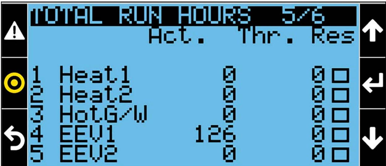
Line #1: Shows the actual Electrical Heater first step run hours counter and the relative settable threshold. If the working hours exceeds this threshold, the El. Heater1 Working Hours Exceeded event will be triggered.
