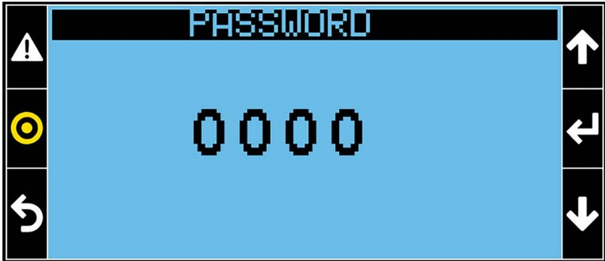
Once one of the three passwords is entered, the user can access the corresponding menu. Higher password levels allows navigation/operation on lower menu level as well. Session will be terminated after five minutes of no key activity. Any time an incorrect password is entered the message “wrong password” is displayed.
