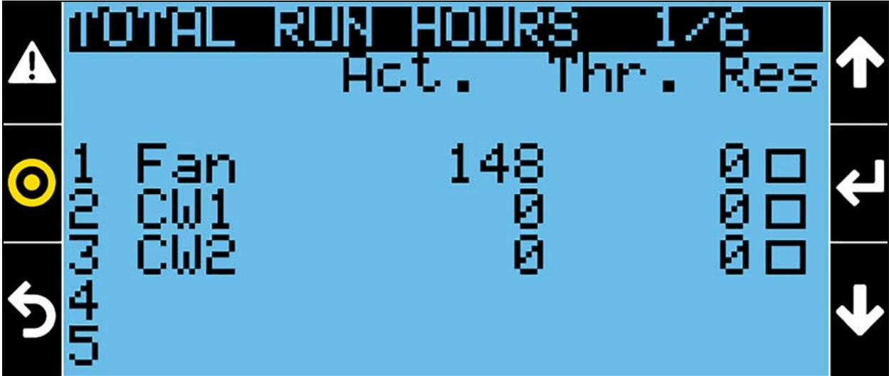
Line #1: Shows the actual fan run hours counter and the relative settable threshold. If the working hours exceed this threshold, the Conditioner/Fans Working Hours Exceeded event will be triggered.
