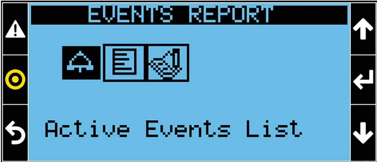
Press the Alarm (🚨) Key to access the Events Report window. A password is not required.
